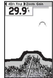
Structure is soft, probably a mud pile
